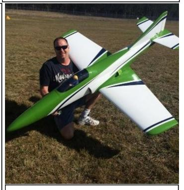
Fuselage is 2.2m long, wingspan 2m. All up weight including fuel and smoke fuel, 17kg. Engine is a Kingtech k140g kero start, 3.5L fuel tank for a 10 minute flight.
