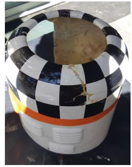
Pull out the plasticine and get rid of any sticking to the cowl with a rag dampened with petrol. This 3M sandpaper is used dry and does not clog up, so goes a long way and worth the extra money.
